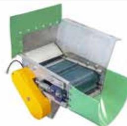
Upper receiving conveyor belt kit, right and left, to direct the harvested product into the destemmers. Made up of a stainless steel frame, 2 rubber rollers, PVC conveyor belt, gearbox and hydraulic motor. The independent movement of receiving conveyor belts and destemmers allows the user to regulate correctly the discharge speed and volume of the products, optimizing the results of the destemming phase.
