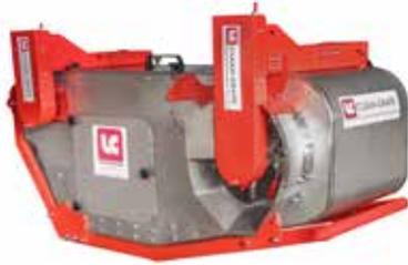
The destemming-chamber isolates the action of the rotor, avoiding it from throwing and then crushing the residuals along the sorting chain, disposing the stalks, stems and leaves quickly. The helicoidal rotor is equipped with techno-polymer moulded extremities, which are delicate on the grapes also at high speeds and in condition of elevated production. The extremities incidence itself and the rotor rpm are easily adjustable to match the features of the harvest.
